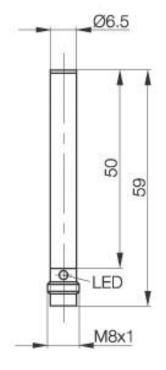
Inductive Sensors BES G06MI-PSC40B-S49G D6.5 x 59 normally-open Sn=4mm quasi shielded
